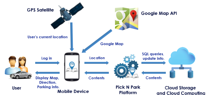
Fig. 2. System architecture of the Pick N Park system.
