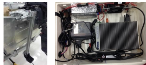
Fig. 7. Garmin 421s echo sounder at the vessel stern (Left); Advantech embedded computer and Novatel GPS inside the electronic box (Right).
