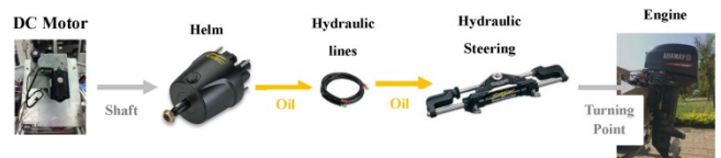
Fig. 2. A connection diagram for hydraulic steering system.
