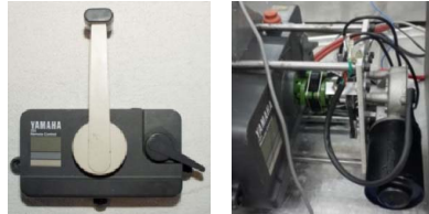
Fig. 5. YAMAHA remote control 701 gear (Left); gear-box of outboard engine connected to the gear servo motor (Right).
