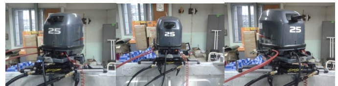
Fig. 3. Hydraulic steering cylinder for the 25-hp outboard engine installed at stern in maximum left-turn position (Left), in center position (Middle), in maximum right-turn position (Right).
